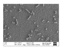
Improved hydrophobic coated (water contact angle: 140°)
